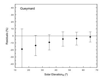
Fig. 2. Residuals of the model in terms of the solar elevation angle.
